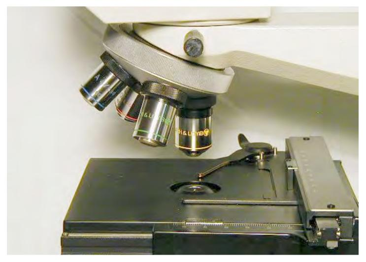
This is a close-up of the lens turret and stage. The lens you need can be rotated into position on the turret. The clip holds the slide in place. The hole in the stage allows light to shine up from below, through the *substage condenser*.
